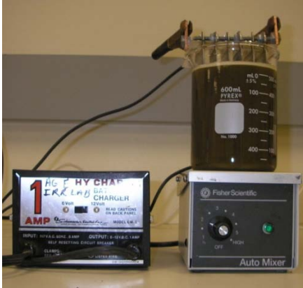
Figure 7.10: Bench-scale EC system with mono-polar electrodes in parallel connections
