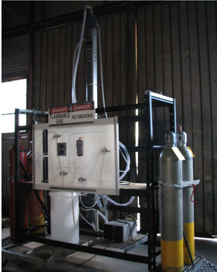
Figure 9.7: Experimental biogas purification set-up.
