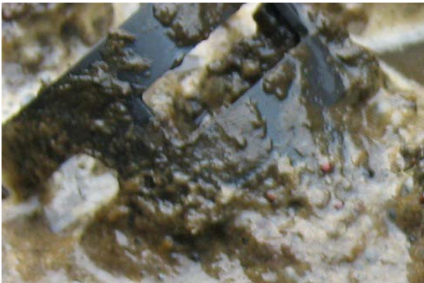
Figure 11.16: Plastic support media with loosely attached biofilm sludge
